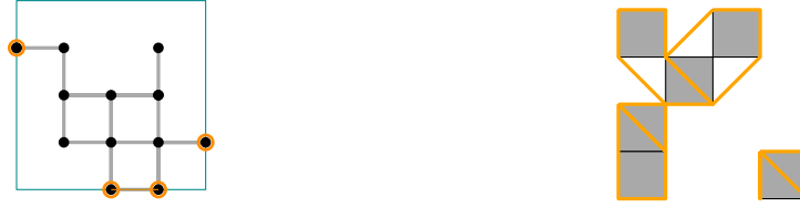
(A) The subset of points stored from a connected component inside a cell. (B) Possible connected components of the grid (black cells are non-empty).
